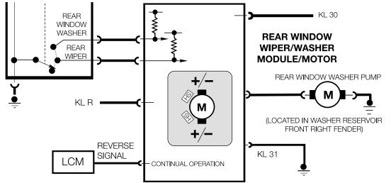
The programmed wiper interval procedure is identical to the E39 sport wagon; Briefly switch the rear wiper ON/OFF, Wait the desired interval time, Switch the rear wiper ON again. The OFF time will be the programmed interval - up to approx. 30 seconds
